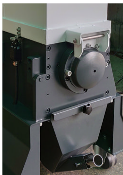
Picture 6-8: Installation of Feed Box, Feed Port and Storage Box 2
