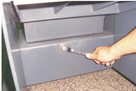
Picture 6-17: Adjustments of V Belts 1
