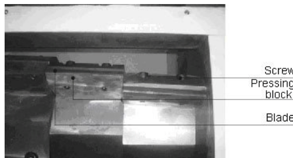
Picture 6-15: Installation of Rotating and Fixed Blade
