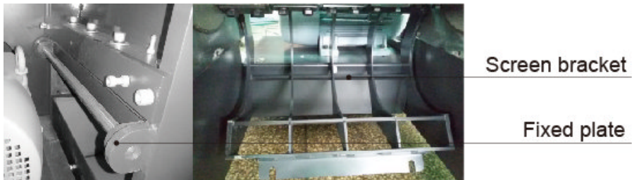
Picture 6-7: Installation of Screen Bracket
