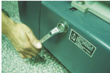
Picture 6-18: Adjustments of V Belts 2
